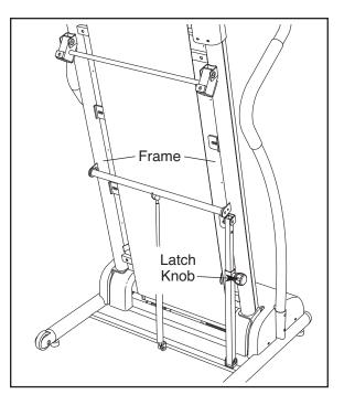
2. Hold the metal frame firmly with both hands and lower it to the floor. CAUTION: Do not grip only the plastic foot rails or drop the frame to the floor. Bend your legs and keep your back straight.
